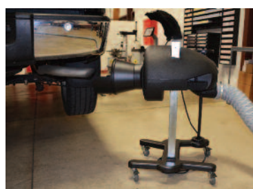
The height position is controlled by a quick-release spring-loaded cam lock.
